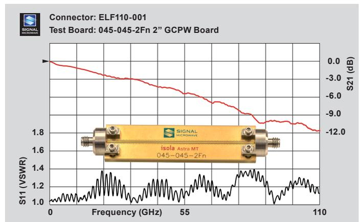
2" GCPW test board with typical data through 110 GHz
