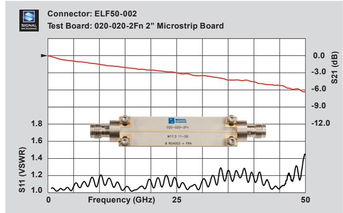
2" microstrip test board with typical data through 50 GHz
