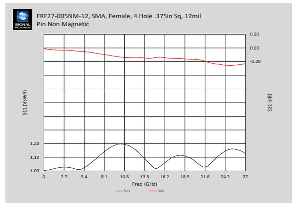
Typical test data through 27 GHz using FRF27-005NM-12 back-to-back connector pair with test pin.
