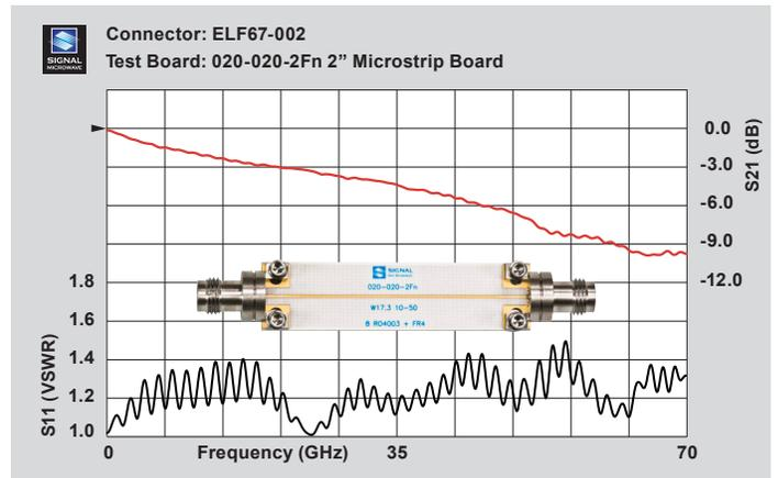
2" microstrip test board with typical data through 70 GHz
