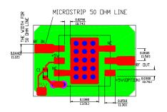
Figure 2 Test board layout for WHM25-1525AE
