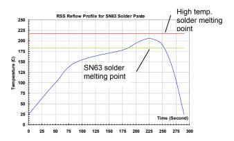
Figure 6 Recommended RSS solder reflow temperature profile.
