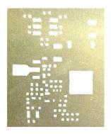
Figure 5 An example of a 0.004" thick stencil.
